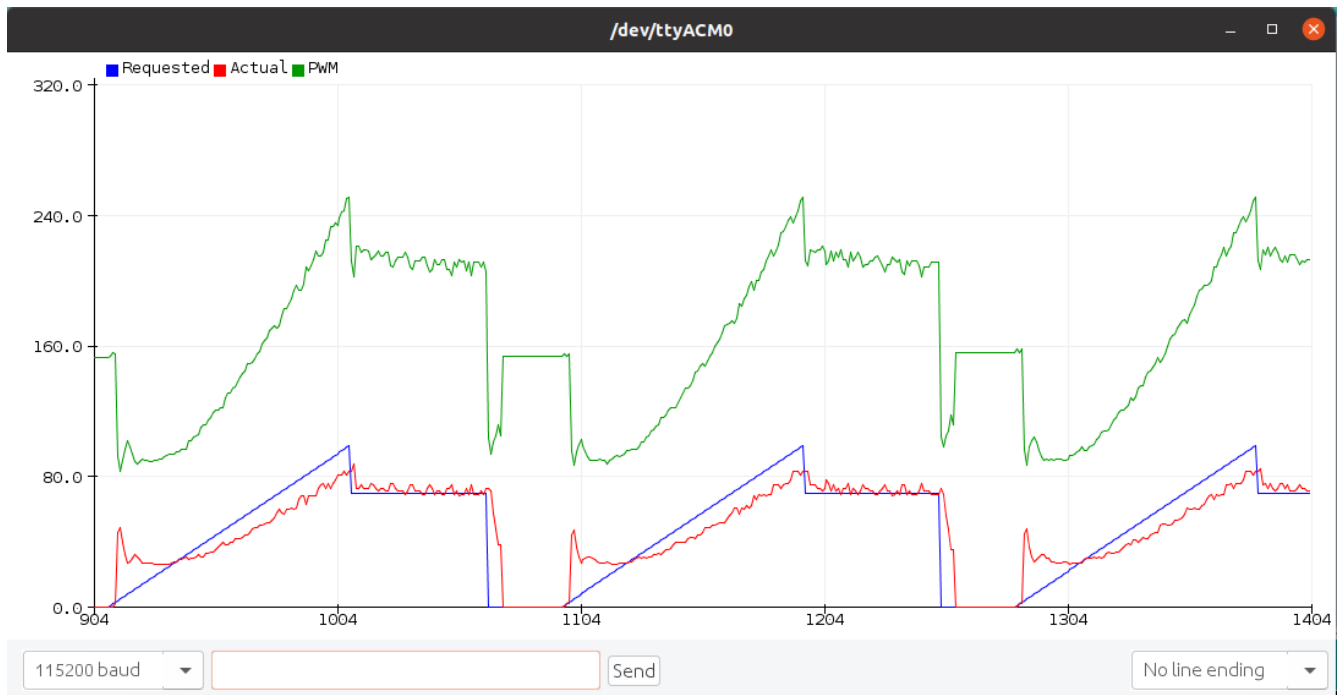
Figure 19: PID control loop results for a complex command pattern
