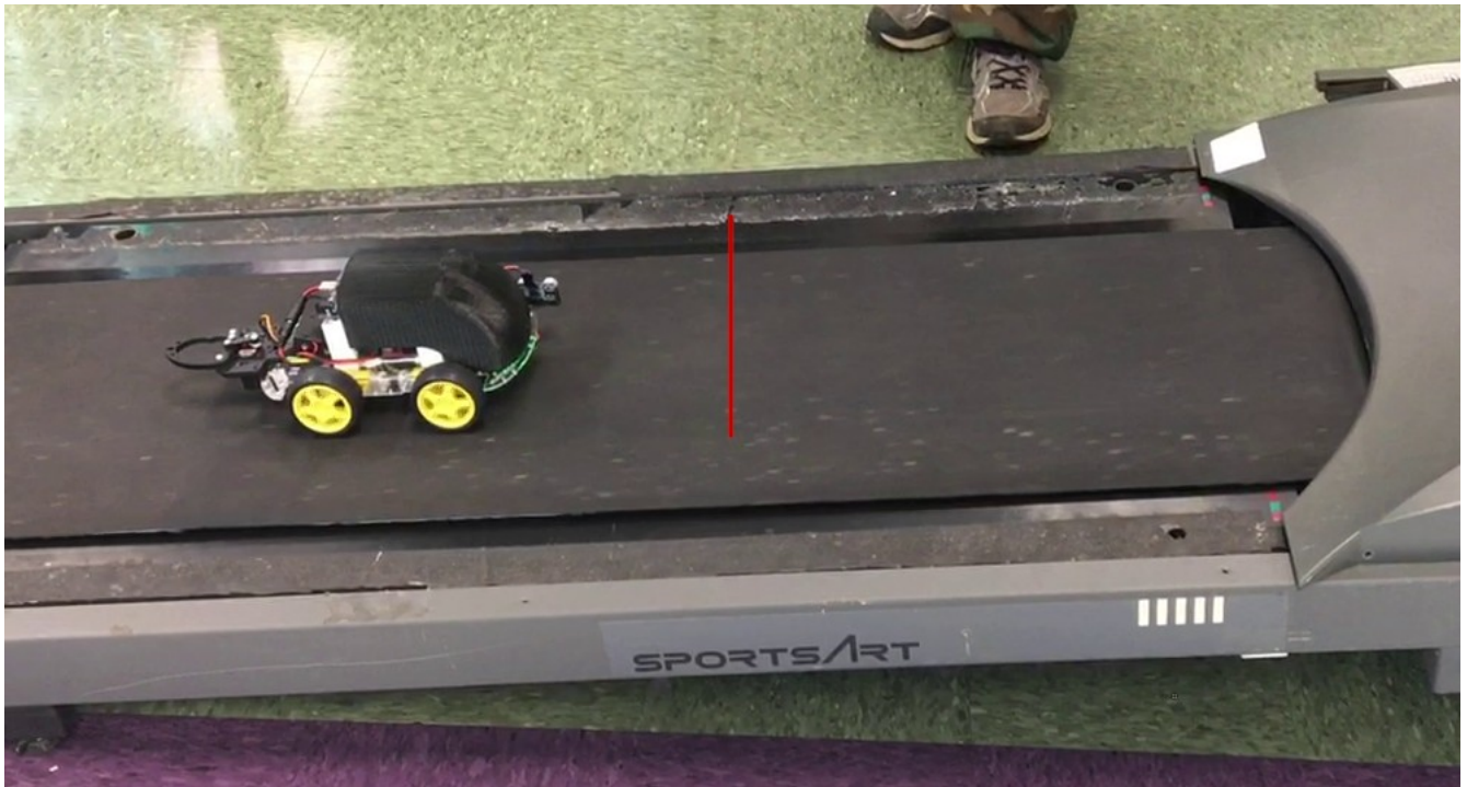
Figure 25: Upper measurement of PID test
