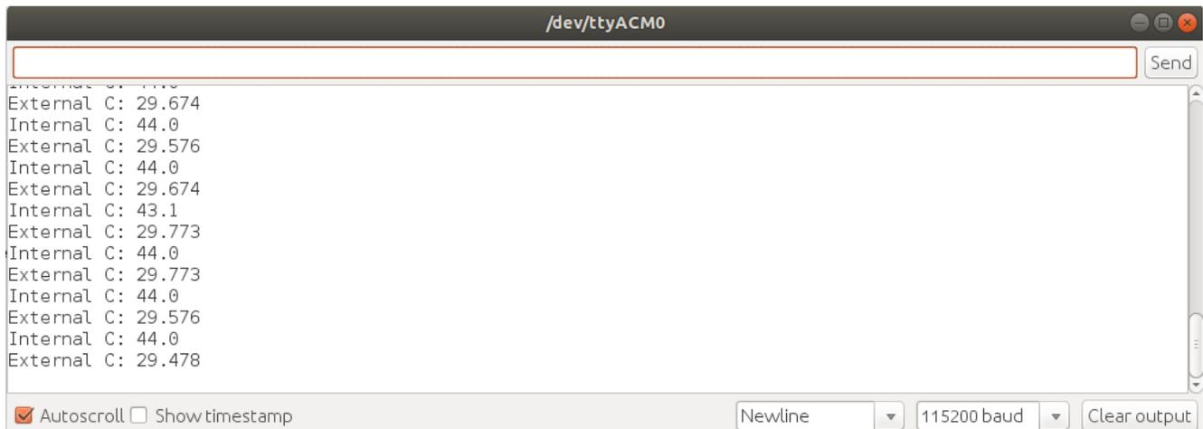
The screenshot shows a Serial Monitor window titled "/dev/ttyACM0". The window contains a list of temperature readings for both external and internal sensors. The external temperature readings are approximately 29.5°C, and the internal temperature readings are approximately 43.1°C to 44.0°C. The window also features a "Send" button, a "Autoscroll" checkbox (checked), a "Show timestamp" checkbox (unchecked), a "Newline" dropdown menu, a "115200 baud" dropdown menu, and a "Clear output" button.
